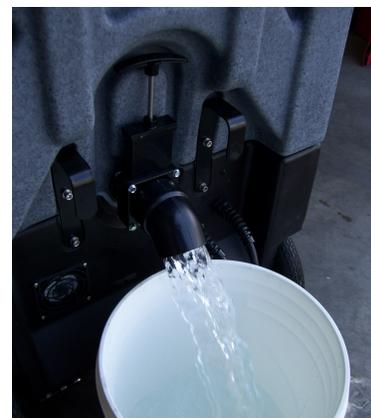
Drain water from Recovery Tank
