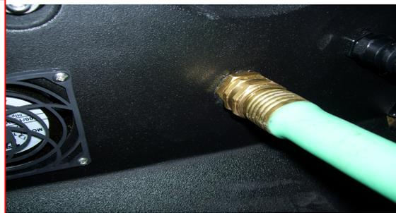
If not using the waste pump-out, the pump-out hose does not need to be connected. When the recovery tank fills during cleaning, the float assembly in the vacuum inlet filter will rise and will automatically shut off the vacuum air flow to prevent the recovery tank from overflowing and waste water from getting into the vacuums. When this occurs:
