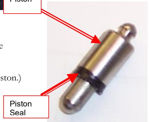
Lubricate Piston Seal with synthetic grease
