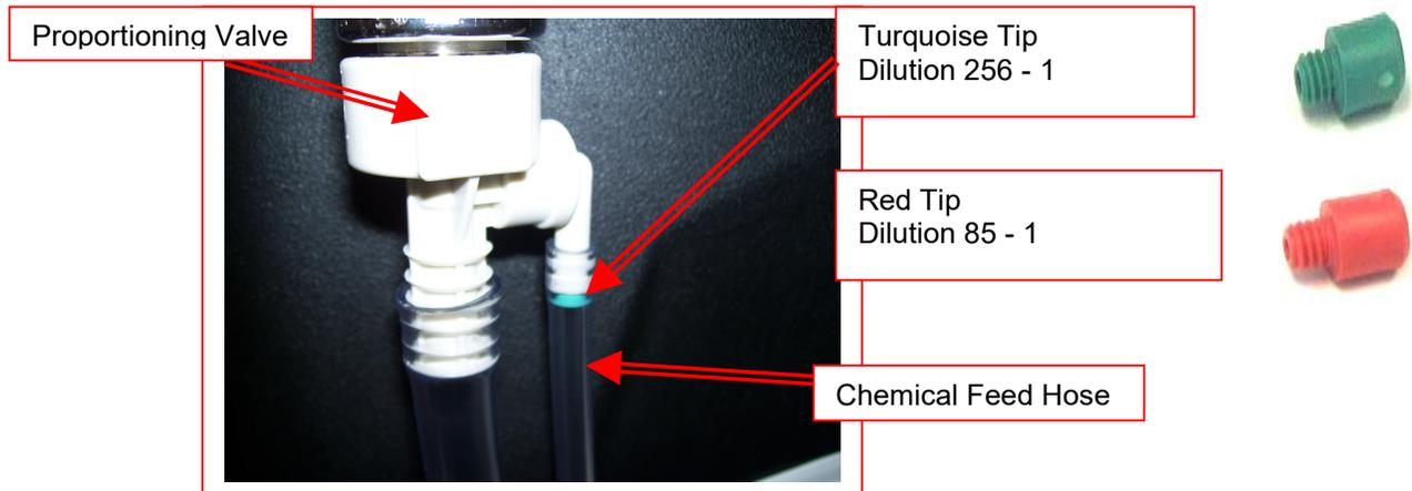
**Metering Tip Kit (Hydro-Force Item# PDE001)** contains 14 different colored metering tips, allowing dilution rates from 11:1 up to 427:1. Refer to the chart below to select the tip that meets the dilution rate for your chemical application.
