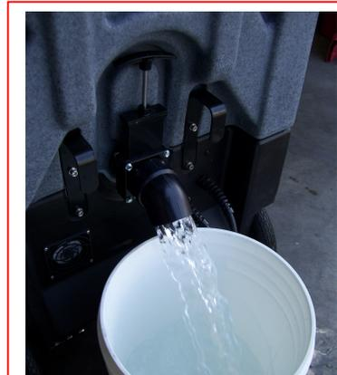
Vacuum acid solution out of Solution Tank
